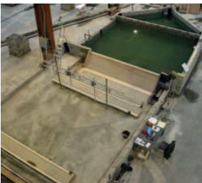
OMAN | AK01 dam - Scale: 1:70 Stepped spillway
