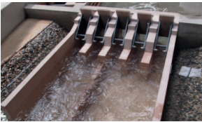
NEPAL | Karnali dam - Scale: 1:100 Gated flood spillway
