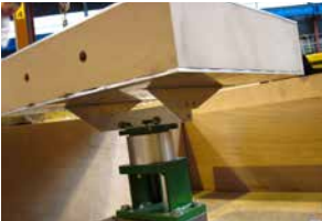
AUSTRALIA | Measurement of hydrodynamic forces on a loading platform
