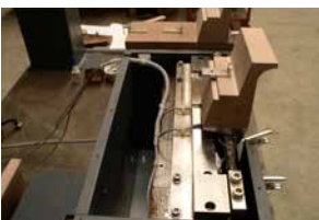
ITALY | Measurement of hydrodynamic forces on a crest wall
