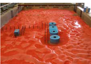
ITALY | Measurement of hydrodynamic forces on a crest wall
