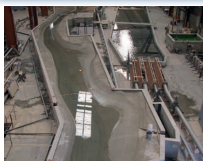
CONGO | Inga 1 & 2 Horizontal scale: 1:100 - vertical scale: 1:140 Sediment removal from the existing structure's head race
