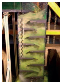
FRANCE | Les Bâteliers model - Scale: 1:15 Flow into the vertical stepped shaft
